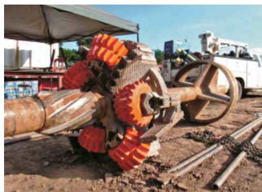
A 48-in. Full Face Hole Opener with milled tooth cutters and 47-in. centering device behind.
