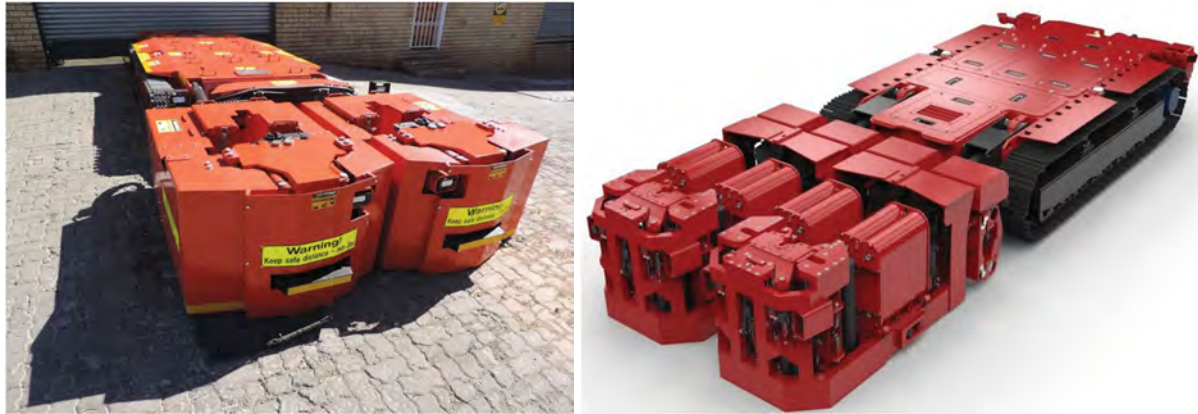
Figure 64: 2014 (left) and 2019 (right) versions of the Minova semi-automated bolter rig (Conner et al. 2020)
