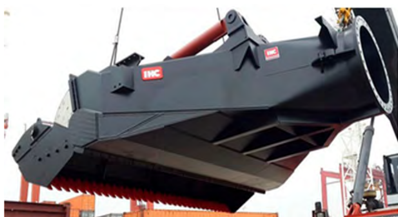
Figure 49: Cutter head for cutter dredge (l) and draghead (www.royalihc.com)
