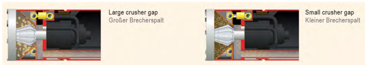
Figure 31: MTS Microtunnelling Systems GmbH – mtsCrushAdjust® grain size control by adapting gap width for the “cone” crusher ( www.mts-tunneling.com/en/ )
