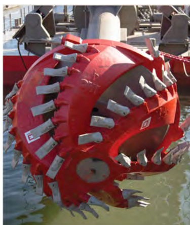
Figure 49: Cutter head for cutter dredge (l) and draghead (www.royalihc.com)
