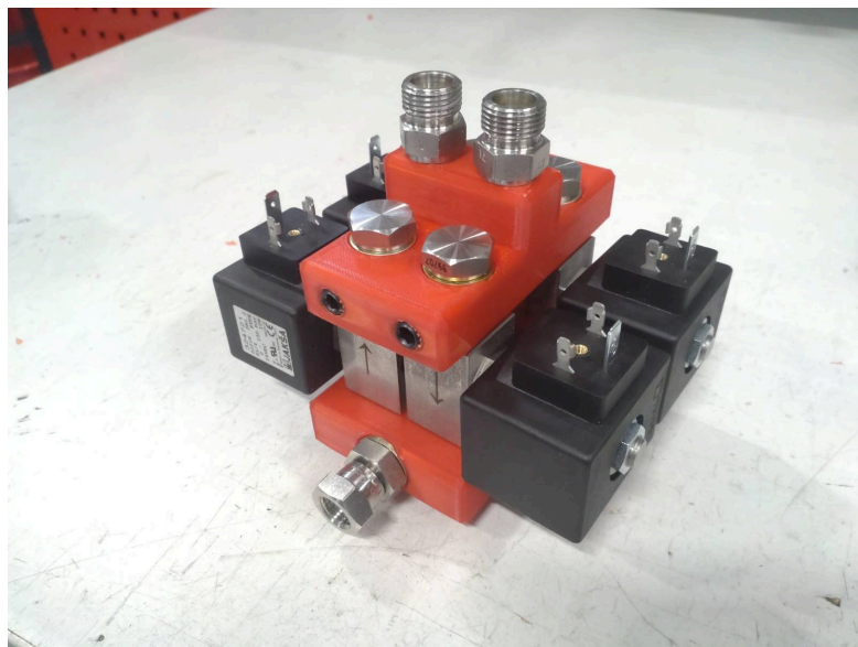
Figure 15 3D-printed mockup of the leg lateral actuator valve block
