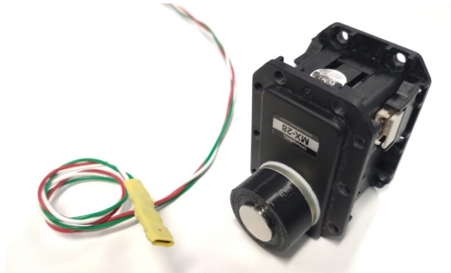
Figure 66 Magnet mounted on a servo motor and the sensor
