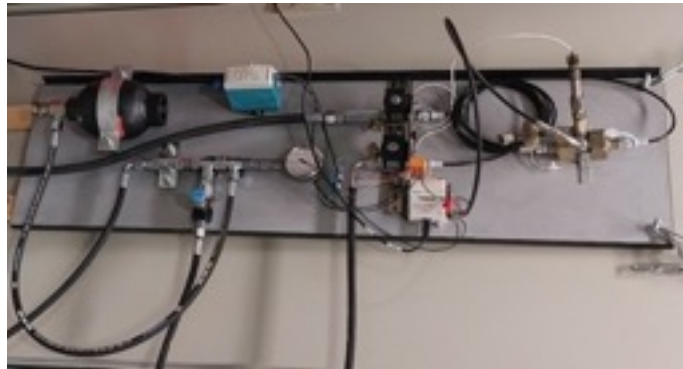
Figure 55 Pressure cycling test system
