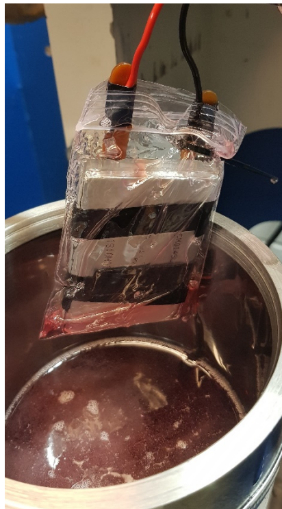
Figure 56 Lithium battery cell after pressurized in oil
