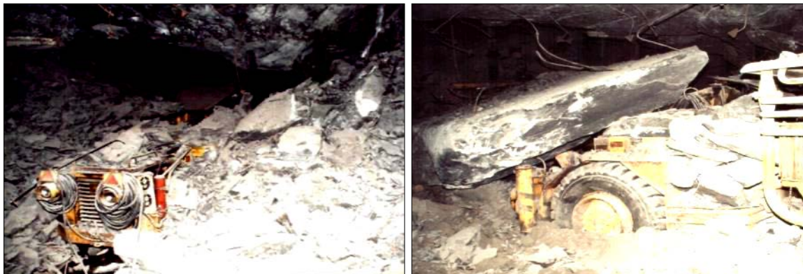
Figure 3.11: Examples of damage resulting from rockbursts.
