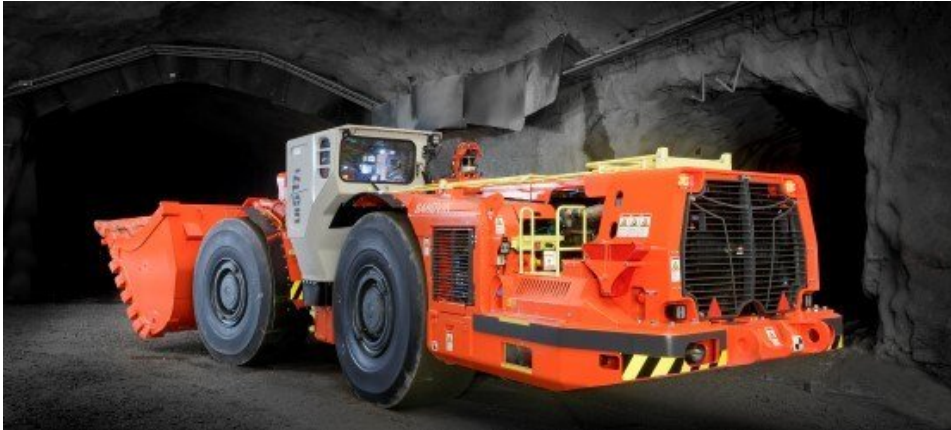
Figure 5.8: Manually operated LHD machine working in an underground mine (Sandvik, 2021).
