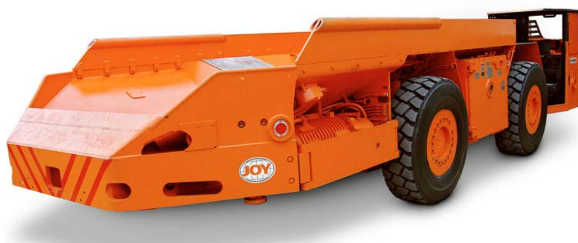
Figure 5.7: Shuttle Car (Komatsu) (Joy, 2021).
