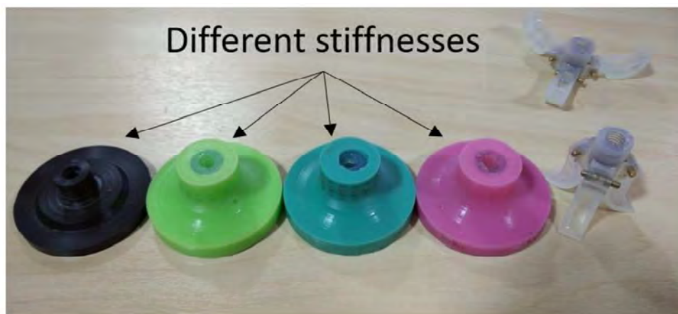
Figure 20 Early feet samples with varying stiffness
