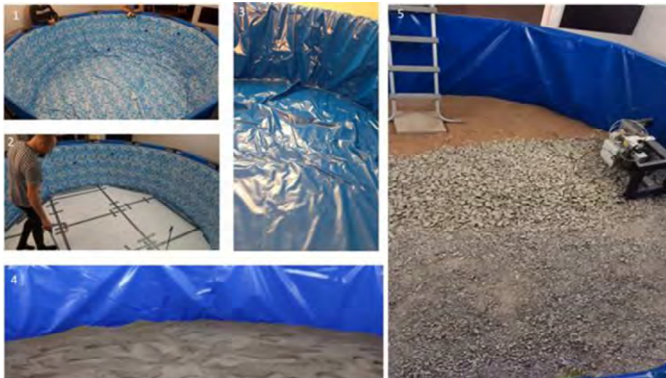
Figure 1 Different pool filling steps and the 5th shows how the mediums are divided inside to the pool
