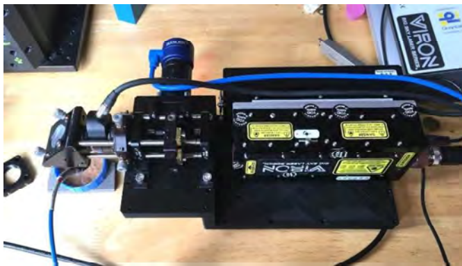
Figure 33 overview of the LIBS instrumental setup tested for ROBOMINERS. Top left: early demonstration platform for solid samples based on a microchip laser (1030nm - 100 \mu J/2kHz). Top right: fiber-laser based prototype (1064nm - 1mJ/20KHZ). Bottom left: slurry LIBS spectrometer, based on a DPSS laser (1064nm - 50mJ 20Hz). Bottom right: plasma spark on a slurry sample.
