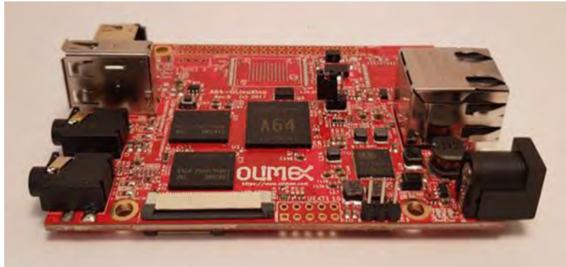
Figure 40 The topside of a single-board computer A64-OLinuXino-1G
