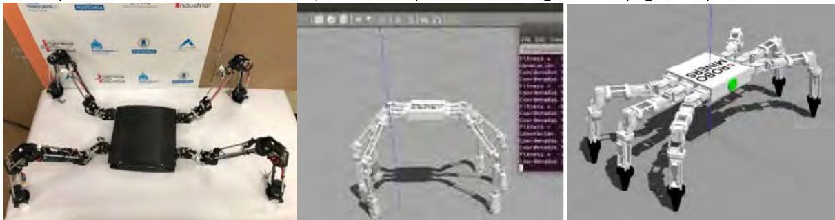
Figure 12 . Early prototypes of modular legged robots. Each leg is a complete robot. Left: physical prototype, right virtual prototypes. Different kinds of gaits and configurations can be created
