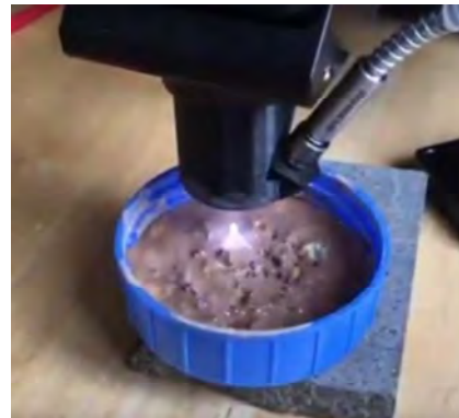
Figure 33 overview of the LIBS instrumental setup tested for ROBOMINERS. Top left: early demonstration platform for solid samples based on a microchip laser (1030nm - 100 \mu J/2kHz). Top right: fiber-laser based prototype (1064nm - 1mJ/20KHZ). Bottom left: slurry LIBS spectrometer, based on a DPSS laser (1064nm - 50mJ 20Hz). Bottom right: plasma spark on a slurry sample.
