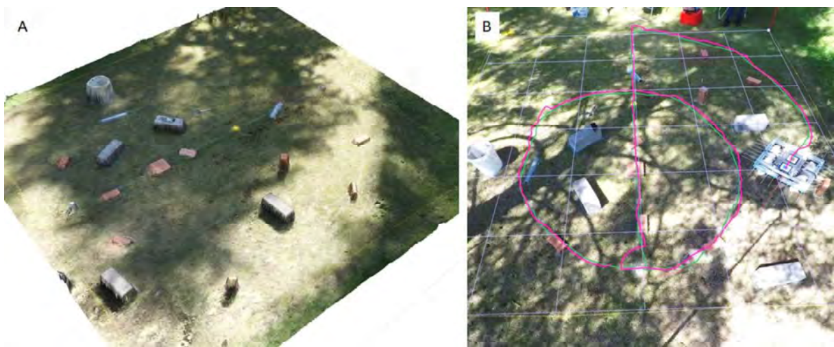
Figure 25 Controlled environment tests. A: reconstructed 3D view of the test ground. B: Camera based tracking of the test platform location
