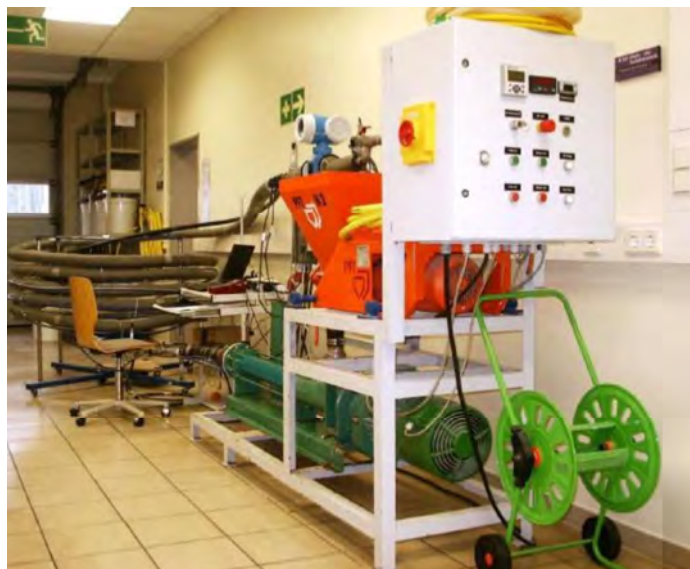
Figure 36 (top) conceptual schema of the LIBS slurry analyser test setup. (bottom) Slurry circulation device at the KUTEC facilities.
