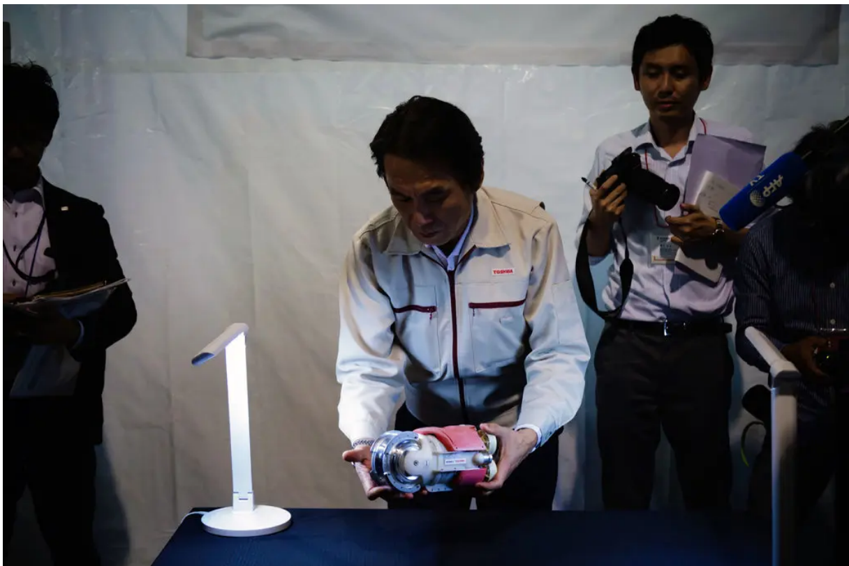
Figure 3: Mini-Manbo (meaning “little sunfish”) at a demonstration in Yokosuka, Japan. It succeeded where previous robots had failed, manoeuvring around debris and avoiding excess radiation to locate the uranium fuel spilled at Fukushima plant. Credits: Ko Sasaki for The New York Times via https://www.nytimes.com/2017/11/19/science/japan-fukushima-nuclear-meltdown-fuel.html .
