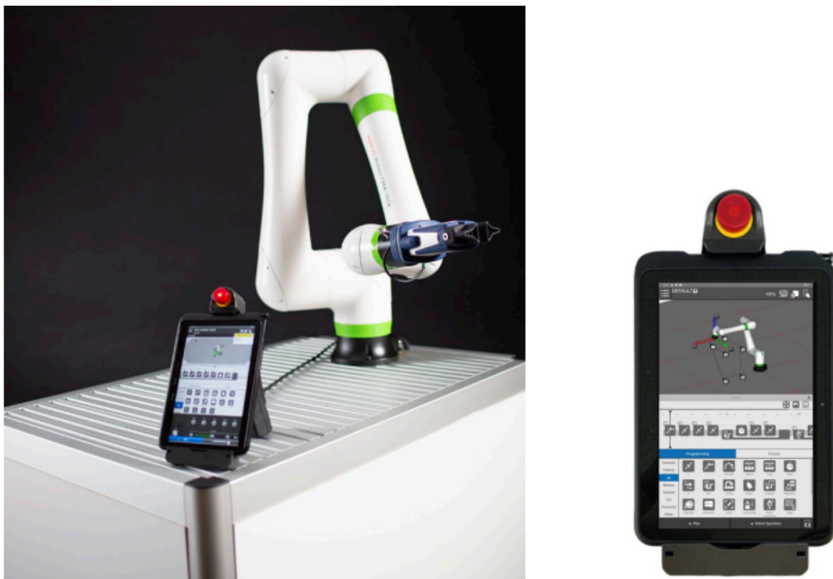
Figure 6: FANUC CRX cobot ("FANUC timeline programming" is shown on the screen of TP). Credits: International Federation of Robotics, via https://ifr.org/img/worldrobotics/Editorial_WR_Industrial_Robots_2021.pdf .
