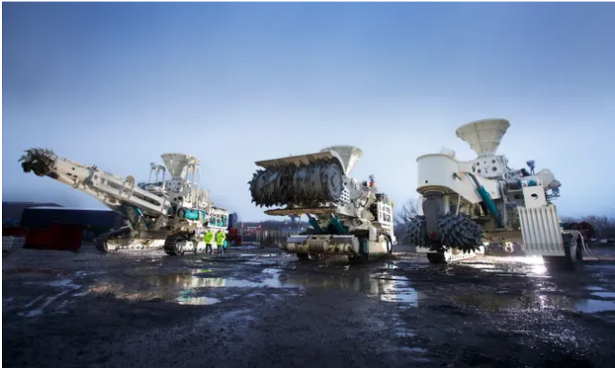
Figure 9: the three Nautilus Minerals robots, built by SMD. Credits: Nautilus Minerals, via https://www.theguardian.com/world/2019/sep/16/collapse-of-png-deep-sea-mining-venture-sparks-calls-for-moratorium .
