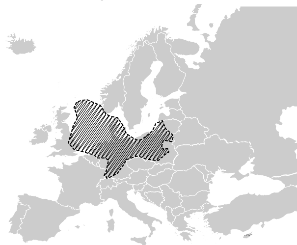
Kupferschiefer*: thickness of 30 to 60 centimetres and maximum 2 metres Depth up to 1,580 metres
