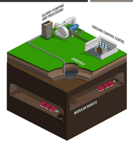
Robot parts (modules) are sent underground via a borehole
